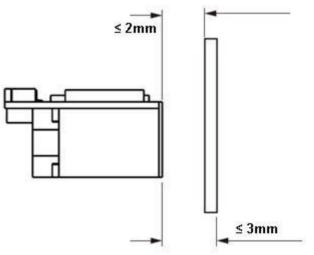
If the window is required to be in a tilted position, the above distance requirements should be met and tilt angle should ensure no reflections back into the lens.
